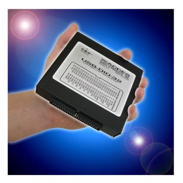
High-Speed USB 2.0 Module Provides 32 Lines of Optimized Digital I/O for Flexible and Economical Digital Control and Monitoring (Model USB-DIO-32)
