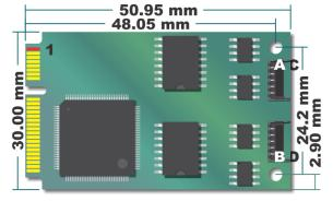
The RS422 ports are terminated by a  $120\Omega$  load in series with a 0.01µF capacitor across the Rx+/Rx- pair.
