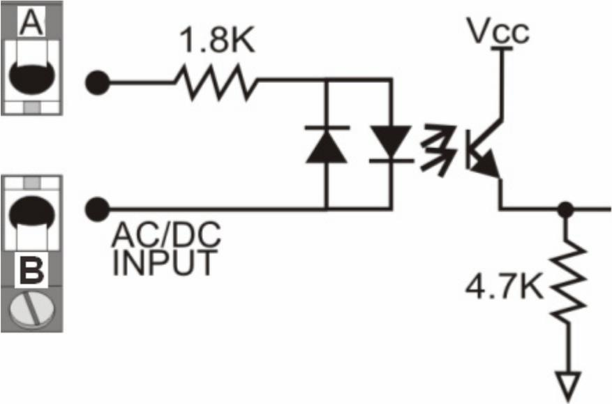
Figure 4-1: Input circuit diagram from screw terminal connections
