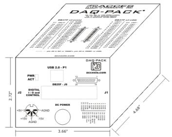
Figure 2-1: DAQ-PACK with one AIMUX-32
