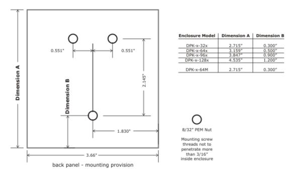
Figure 2-2: DAQ-PACK Mounting Provisions
