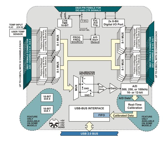
Figure 1-1: Block Diagram
