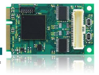
It uses the high speed PCI Express bus to transfer digital data to and from the card. The digital I/O is compatible with 8255 PPI chips making it easy to program. This allows for simple and trouble-free migration from other ACCES PCI and PCI Express digital I/O cards, but also provides for advanced features enabled by the onboard FPGA logic.
